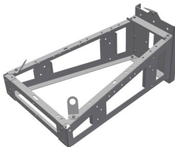
2. Tightening torque should be not less than 40 Nm
