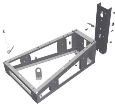
1. Fasten the pole interface bracket and lifting provisions
